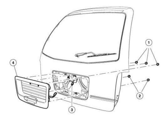
3. To install housing, reverse the removal procedure.
