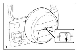
c. Detach the 8 claws and remove the spare wheel cover.
