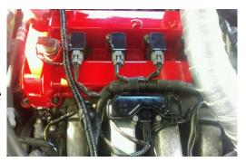
Make sure you have enough clearance below your charge piping. You should have at least ¾" to 1" of clearance above your ignition coils. If you don't, you will need to reposition your couplers or shim your upper charge pipe mounting bracket with washers.
