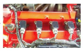
Insert the engine cover (4) bolts into the coil mounting holes. Start all 4 socket head screws by hand and then tighten with a 5mm allen wrench. Bolts should be tightened up snugly but be careful to not over torque them.
