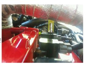
Remove your upper charge pipe (if applicable) Remove all 4 ignition coil bolts (these will not be reused)
