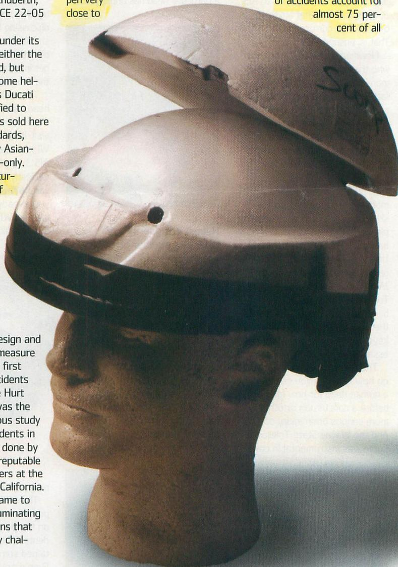
All the Snell/DOT helmets we examined use a dual-density foam liner. The upper cap of foam on this Scorpion liner is softer to compensate for the extra stiffness of the spherical upper shell area. Some manufacturers, including Arai and HJC, use a one-piece liner with two different densities molded together.
