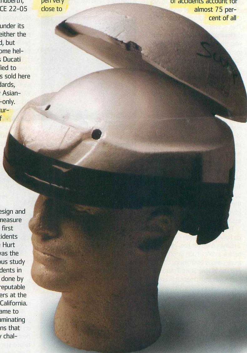
All the Snell/DOT helmets we examined use a dual-density foam liner. The upper cap of foam on this Scorpion liner is softer to compensate for the extra stiffness of the spherical outer shell area. Some manufacturers, including Arai and HJC, use a one-piece liner with two different densities molded together.
