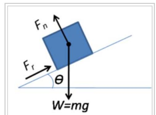
Weight ( $W$ ), the frictional force ( $F_r$ ), and the normal force ( $F_n$ ) impacting a cube. Weight is mass ( $m$ ) multiplied
