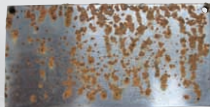
After 192 hours in a humidity cabinet, the metal coupon treated with a leading competitive product rusted severely.
