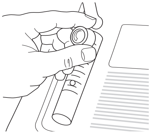
Using a flowmeter liter control knob to adjust the oxygen flow rate
