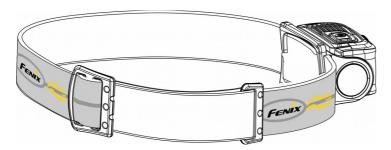
Slide the plastic buckle to adjust the headband.
