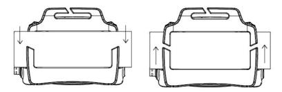
Attach the headband to the headlamp as shown by first sliding the band down to the bottom of the slot, then hooking the top edge under the top slot.
