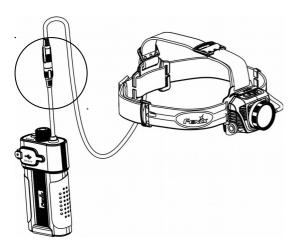
Plug the cable from the headlamp into the connector of the battery box. If additional stability is needed, attach the top headband to the headlamp holder and the top headband mount as shown.
