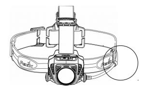
Use the clips supplied and the cable slot at the top headband mount to retain the battery cable.
