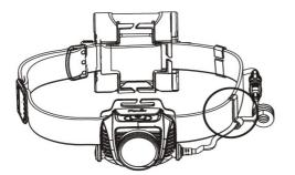
Use the clips supplied to retain the battery cable.
