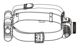
If additional stability is needed, attach the top headband to the headlamp holder and the battery case as shown.
