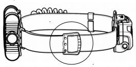
Slide the plastic buckle to adjust the headband.
