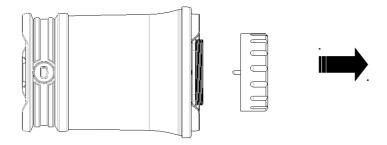
Unscrew the battery cover counterclockwise
