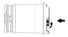
Put the battery cover back on and screw it clockwise to secure it
