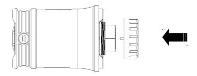
Insert the battery with the anode side (+) toward the light's head
