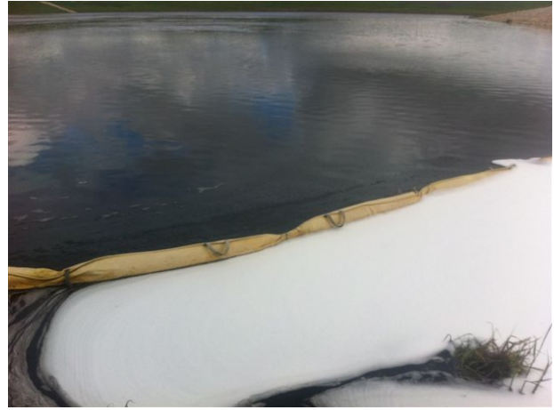
The Froth Cap spreads over the oil slick, over rocks and between grasses.
