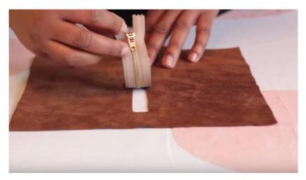
Step 2— Stitch the zip in place. This can be done on a machine with a leather needle and ideally a walking foot, or else by hand, using a chisel or awl.
