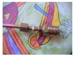
This fitting was a bit harder to find but it was a good find. It adapts the 3/16" copper pipe to a 1/4" air fitting using compression. You slide the top and the little ring over the pipe. Stick the pipe in the fitting and screw it on tight. Easy peasy!
