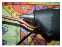
You want to bend the pipe so that it is parallel to the tip of the gun. You will want to play with this later though to get a good blowing result. Cut the pipe off flush with the end at a slight up angle to the tip.
