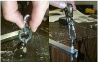
Now you can connect the swivel pulleys using the quick connects. Note that the picture on the right shows the installed pulley on the BOTTOM of the end of one arm (frame is lying upside down) (1) pulley on each arm end and (1) on the bottom center eyebolt of rear frame.
