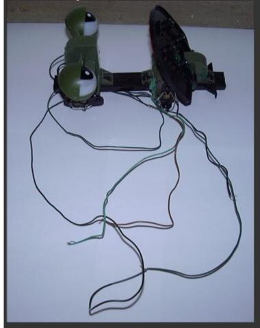
Now all you have to do is strip the ends of the wires, and then make your connections. You will either be hooking it up to the end of an RCA jack cord or just two sets of wires, whatever your stereo uses for speaker output. So depending on what type of connection you have, you can skip to the section explaining each and follow those instructions.
