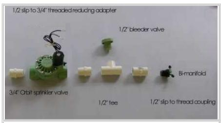
This is a picture of the parts needed for the sprinkler manifold that will be constructed at the Manifold workshop. This list consists of (from right to left)
