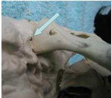
Bucky's jaw is held in place by a pair of springs. We need to install a permanent pivot for the jaw and also eliminate the springs because they are too much mechanical resistance for the servo. We'll use the cable ties as our pivot. Using a drill bit the same size
