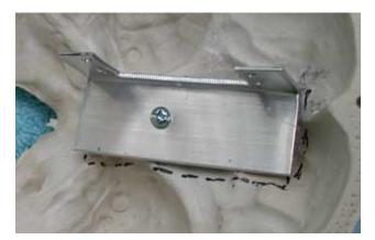
Using the #6screw, nut and washer , mount the servo bracke t in the Bucky skull. Tighte n securel y but don't over
