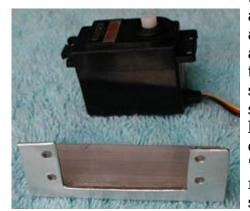
Using the appropriate tools (hack saw, tin snips, file, etc.) cut an opening in one side of the aluminum angle to accommoda te the servo. Be sure to leave some of the "angle" to maintain strength. Drill holes to match the servo mount for 4/40screws. This will be our servo bracket.
