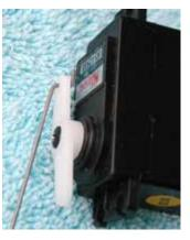
Feed the wire through the hole and install the servo in the bracket using the #4/40 screws and nuts. I find that using just two screws will hold it securely in place.
