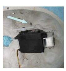
While holding the servo in place, make a mark on the skull in line with the two points described above (left). Drill a 1/4" hole in the skull at this mark. If you were really good (lucky?), the hole will line up perfectly between the two points, if not, you'll have to "modify" the hole slightly to be in line.
