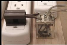
Shown is a 120V, 4 Pole, Double Throw, KH style or "Ice Cube" relay. Nicknamed that since these relays are always covered with clear shells so you can actually see inside. That must be for geeks like me that have to see it before I can understand it. I work with these as they are readily available from surplus places such as All
