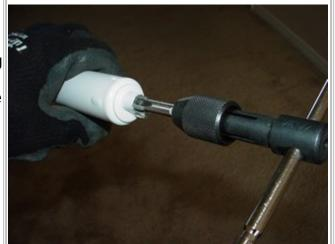
Once I had the end of the piston threaded I test fitted the elbow that I picked up while on my search for parts.
