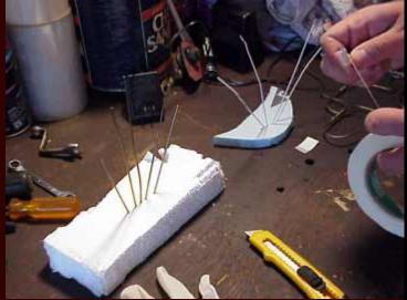
Next I used packing tape and wrapped it around the wire to make the knuckles and give the fingers some width.
