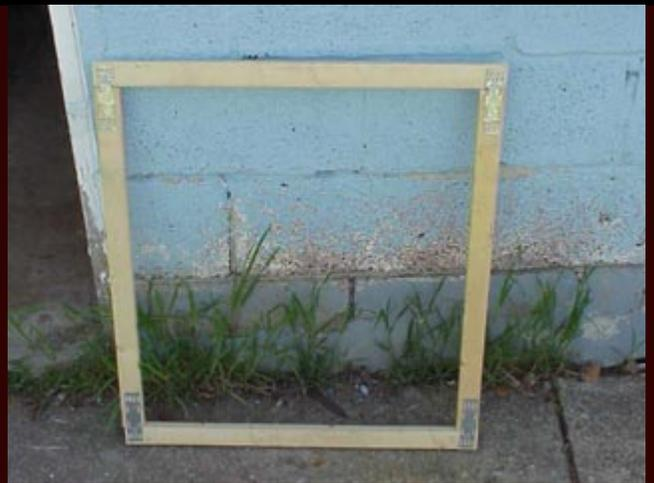
Here are both ways we used for connection. If you want to do it quick, use the metal straps. If you want to do it cheap, use screws. Remember if you use screws anywhere in the project you must drill pilot holes.
