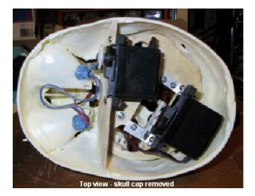
The photo below shows some detail of the jaw servo mechanism. The servo wheel is attached to the jaw using ball joints and threaded rod which can be obtained from any good R/C supplier. The ball joints allow both ends of the rod to move freely -
