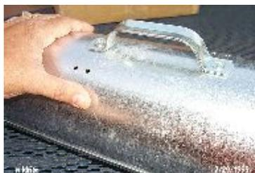
The handle is just bolted on top. You can also see a couple of coil support holes here.
