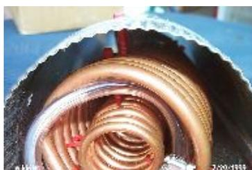
If you look closely, you can see how the coils are suspended inside the stove pipe. I used red plastic wire ties to connect the inner coil to the outer coil, and a second set of ties to connect the outer coil to the stove pipe.
