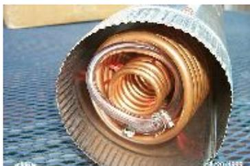
This is what the end of the chiller looks like. You can see the 1.5 inch inner coil and the 3 inch outer coil and the short plastic tube connecting them.
