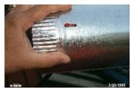
Here you can see how the ties connect to the stove pipe. I drilled two small holes for each tie and then just looped the tie through one loop of the coil and through the holes. Start by leaving the loop loose, and attach the coil at three points around the stove pipe, then tighten the loops a bit at a time till the coil is in the middle. Do this at both ends and add a few in the middle. You may have to get your kid to do the inner one. My hand was too big!
