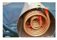
This is the other end of the chiller. The red caps came on the copper I bought. You remove them and that is where the plastic tubing is attached. I drilled some larger holes for the tubing to exit that you can just barely see on the top of the stove pipe.
