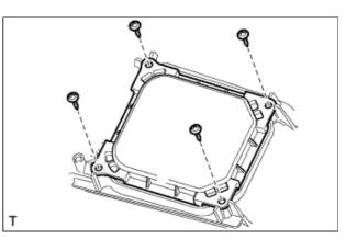
Disconnect the connector and remove the headlight light control ECU subassembly.
