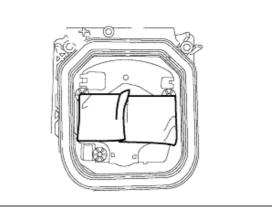
e. Remove the headlight reflector LH as shown in the illustration.
