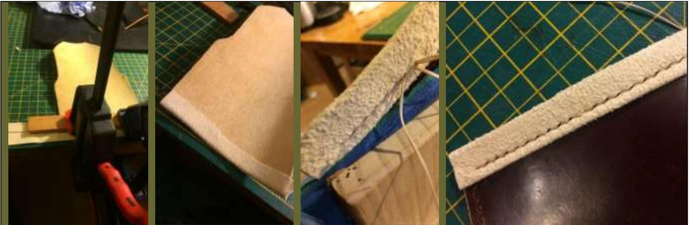
The next step was to glue in place the seam over the edge, and again clamp with an even amount of pressure whilst the glue set. Once it had set, I marked out a stitch line the length of the seam, clamped it up in the stitching pony, and saddle stitched the whole seam in place.
