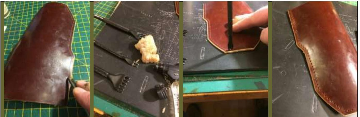
I marked where the stitch line was going to go, and then set about marking out the stitch holes. I used stitching chisels here, marking the holes initially, before tapping all the way through. I started from the first defined corner in the stitch line and worked upwards toward the top of the neck. This made sure that there was a stitch hole where the line changed direction.
