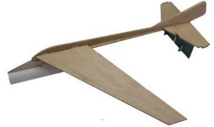
**11.** Attach the wings (5) to the Keel by gluing the tabs in the slots and resting the wing on the Fuselage top. Support the wings in place and make sure the tips just touch the table. View the assembly from the front and make sure both wings form a symmetrical pattern and the pylon is vertical. Some masking tape at the tips of the wings will help support them while they dry.
