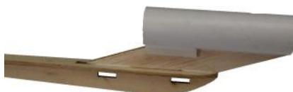
**10.** In preparation to installing the wings, invert the Fuselage/Pylon assembly and support the stabilizer end on the Fin Alignment Tool. The Body Tube should be flush with the table.
