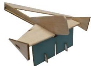
**13.** Run a thin fillet of glue along all the joints. Do not add too much or the increase in weight will affect the performance. After all the glue is dry, sand all the edges round on all balsa parts, except the main wings. Sand them to an airfoil shape for best results.
