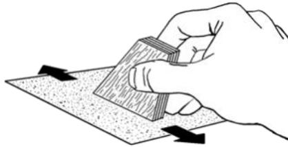
4. Round the leading and trailing edges of each fin. Leave the tip and root edges flat. Repeat for all six fins. The trailing edge can be sanded to a bevel for a more aerodynamic shape. The root edge will be glued to the body tube.
