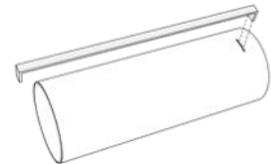
9. Carefully punch out the two fiber rings (RA-5055S). Align the ring with the small slot about 1/8" from the top of the engine hook.
