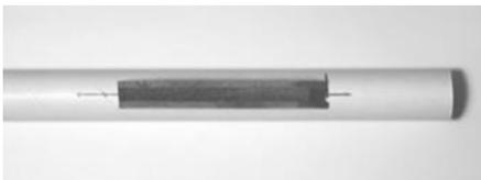
❑ 19. Glue the launch lug into place between the motor pod tube and the pod hook.
