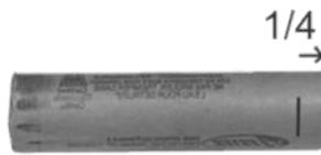
❑ 22. Insert the motor block as shown and push into place with the empty casing until the 1/4 inch mark is even with the end of the tube. Quickly remove the motor casing with a twisting motion.
