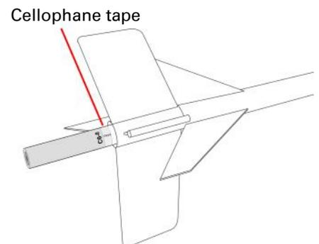
7. Wrap a layer of masking tape around the bottom of the second stage motor and the exposed portion of the second stage motor mount tube. Be careful to avoid overlapping the cellophane tape wrapped joint between the two motors or the stages may not separate!
