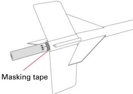
8. Slide on the first stage, then wrap masking tape around the bottom of the first stage motor and the exposed portion of the first stage motor mount tube.
