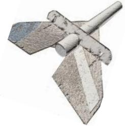
**12.** Remove the masking tape and fold the flaps carefully to crease the hinge. Pop out the Vertical Stabilizers from the balsa sheet and glue them to the Main Fins. The Stabilizers with the notch in the leading edge go on the same side as the hinge. You can use the fin alignment tool to hold the stabilizers in place.
