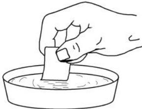
**38.** Slide the decal in place and use the paper backing to work the bubble out. Repeat for all the decals.
