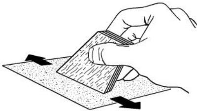
**4.** Repeat for all three sets of fins. Round all leading edges. Round or taper all trailing edges. Leave the tip and root edges flat. Use the diagram to identify edges and fin types.
