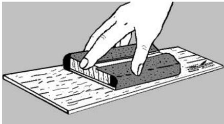
3. Stack all four fins in a group. Line the group up squarely and sand the fins back and forth over some fine sandpaper to get rid of the hold-in tabs as shown below.
