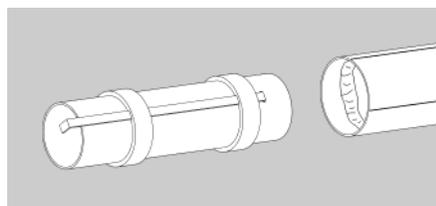
❑ 14. Quickly and smoothly push the engine mount into the marked end of the body tube until about 1/8" is extending from of the body tube and the **engine hook is centered between two of the lines**. Do not stop once you start inserting the mount or it might freeze in place too soon.
