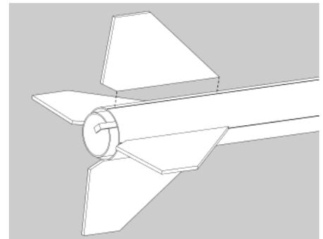
❑ 16. After the fin assembly is completely dry, run a very small bead of glue along both sides of each fin-body tube joint. Using your forefinger, smooth the glue into fillets. Since this is a scale model, it should not have fillets showing. Wipe any excess glue and allow to dry.
