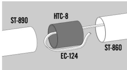
❑ 12. Roll the assembly on a smooth flat surface while the glue sets to get the tubes aligned. Make sure the joint is smooth and the two tubes are touching. Wipe any excess glue and wait for the joint to dry completely. Make sure the elastic is still hanging out of the top of the body tube.
