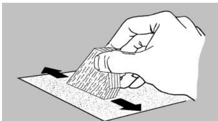
4. Sand a taper on each leading edge .21" wide and leave all the tip and root edges flat. For scale fins, sand to .05" thick.
