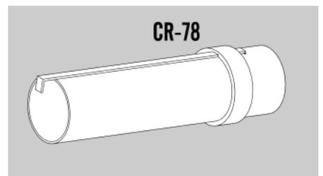
❑ 9. Slide the remaining centering ring (CR-78) over the bottom end of the engine tube. Space it 3/4" from the bottom of the engine tube. Apply a bead of glue around both sides of the centering ring.
