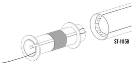
❑ 13. Quickly and smoothly push the engine mount into the marked end of the body tube until about it is even with the bottom of the body tube and the **engine hook is centered between two of the lines**. Do not stop once you start inserting the mount or it might freeze in place too soon.
