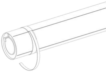
❑ 18. Apply a very thin bead of glue to the dull side of the other band on the widest half. Starting the wide end on the same marked fin line as the lower band, and even with the top of the body tube, apply the band the same as the lower band.
