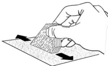
4. Sand a taper on each leading edge and trailing edge and leave all the tip and root edges flat.
