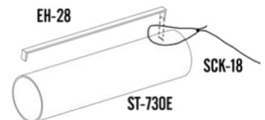
7. Apply a small bead of glue around the inside of the engine tube nearest the punched end. Slide the thrust ring (TR-7) into the tube and against the engine hook.
