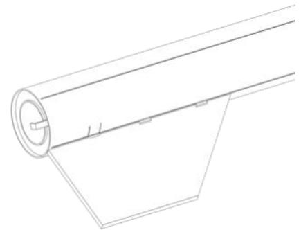
❑ 16. Apply a very thin bead of glue to the dull side of one of the bands (IKD-4S) on the widest half. Starting the wide end on the marked fin line and even with the two marks, carefully wrap the first half of the band around the body tube. The wide ends should meet at the fin line.
