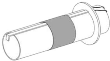
❑ 10. Slide the centering ring with the long slot (CR-KD-4B) over the end of the engine tube. Space it about 1/16" from the bottom of the engine tube. Apply a bead of glue around both sides of the centering ring, keeping glue away from the engine hook and the notch.
