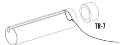
8. Slide the centering ring with the small notch (CR-KD-4A) over the engine tube until it is against the Kevlar cord. Apply a bead of glue around each end of the joint between the ring and engine tube, keeping glue off the outside surface of the centering ring. Allow to dry.
