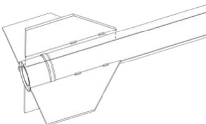
❑ 20. After the fin assembly is completely dry, run a very small bead of glue along both sides of each fin-body tube joint. Using your forefinger, smooth the glue into fillets. Since this is a scale model, it should not have fillets showing. Wipe any excess glue and allow to dry.
