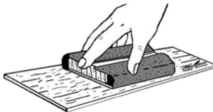
3. Stack all four fins in a group. Line the group up squarely and sand the fins back and forth over some fine sandpaper to get rid of the hold-in tabs as shown below. Sand the root edge **very gently**.
