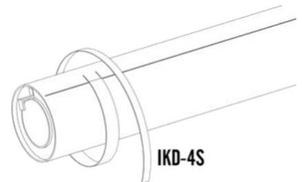
❑ 17. Apply a very thin bead of glue to the dull side of the narrow end and continue wrapping the rest of the band around the body tube, centering the narrow strip over the wide portion. The end should also meet over the previous joint.
