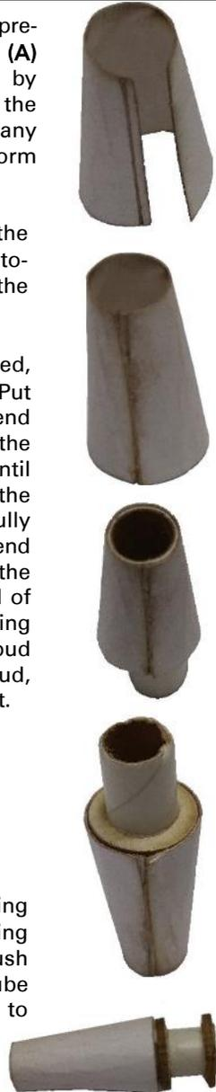
❑ 5. Tie the Kevlar Shock Cord (D) to the Thrust Block (E). Make sure the knot is tied securely. After you have the cord tied, glue the Thrust Block into the end of the Motor Tube with the Centering Rings. Push the Thrust Block in until it is flush with the end of the Motor Tube as shown at right.
