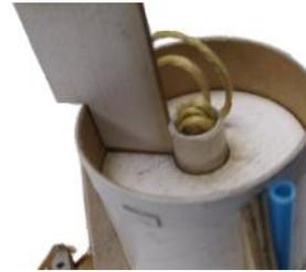
❑ 15. After the Motor Mount has cured sufficiently remove the shock cord from the motor tube and glue the Stuffer Tube (N) to the top of the Motor Tube. The Stuffer Tube should slide over the end of the Motor Tube and rest against the Upper Centering Ring. Add a fillet of glue around the Stuffer Tube to seal and hold the tube.
