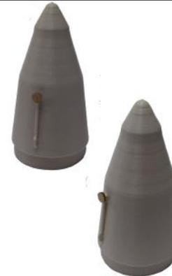
❑ 17. Tie the Shock Cord to the small loop in the Nose Cone. Make sure the cord is firmly attached. Take the piece of Streamer Material (Q) and cut it in half lengthwise so it is 1/2 inch wide. Once you have the streamer cut to width, secure one end of the Streamer to the Shock Cord with Masking Tape as shown at right.
