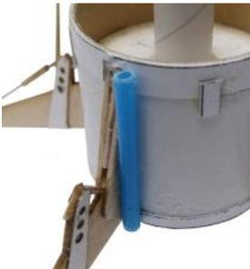
❑ 13. Using Medium Cure Super Glue, attach the Launch Lug (M) to the body tube next to one of the Leg Supports. Center the Launch Lug between the top and bottom of the body tube
