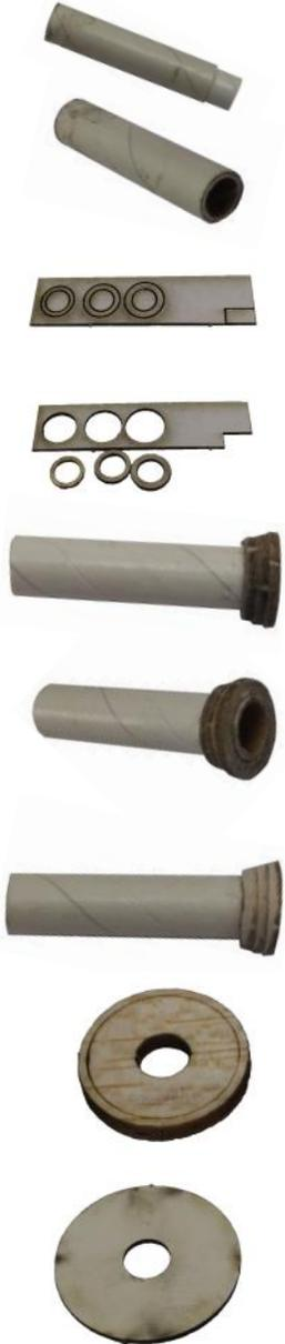
the Base Disk. The Base Disk needs to be beveled to the line on the disk. Again use a file or sandpaper to shape the disk so that it has a taper from the edge to the line as shown in the picture at right.
