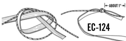
❑ 24. Assemble the chute (CP-12-24) using instructions provided with it. Pull the lines tight on the chute and make sure they are all of equal length. Attach the chute by tying them to the screw eye. Put a drop of glue on the joint to keep the lines from moving. Attach the free end of the elastic cord to the screw eye. Put a drop of glue on that joint as well.
