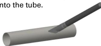
5. Insert the top end of the engine hook through the loop in the Kevlar cord and into the engine tube at the punched slit.
