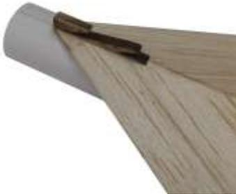
❑ 30. Glue the two Side covers (K) onto the sides of the Glider Hook. Apply glue sparingly so as not to get glue down into the teeth of the hook.
