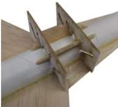
❑ 20. Glue a Wing Fence (7) to the top of the wing in the open slot closest to the body tube. Add glue fillet for added strength when glue has had time to dry. Allow glue fillet to dry. Repeat for other wing.
