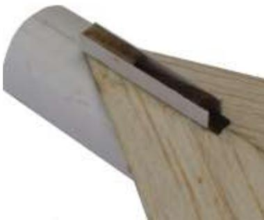
❑ 31. Using the Alignment Jigs, glue the Elevons (13) to the back of the wings. Keep the outside edges even with the edge of the wings.
