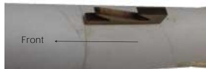
❑ 23. Insert the Screw Eye (L) into the bottom of the Nose Cone (E). Remove the Screw Eye and fill the hole with glue and then re-insert the Screw Eye back into the hole. The glue will help keep the Screw Eye from coming back out.
