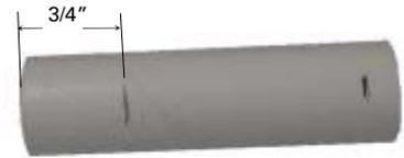
5. Cut a notch 1/32" deep and 3/32" wide on the inside of one of the centering rings (G). This will allow the ring to clear the engine hook.
