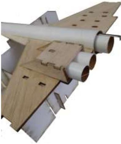
❑ 18. Glue the Wing Tips (3) to the Wings. Use one of the small fiber tools to make sure the wing tips are square with the wings. Once the Tips have had a chance to dry for a little while, go back and apply a glue fillet to add some extra strength to the joint.
