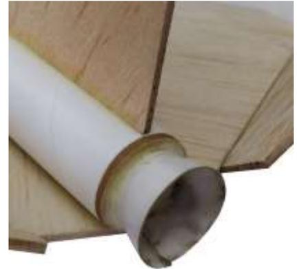
❑ 36. Insert the Nose Cone into the front of the glider body tube. **Do Not Glue at this time.**
