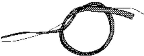
❑ 4. Tie the other end of the yellow Kevlar cord to the thrust ring. Place the elastic cord through the **body tube**. **The thrust ring is to be glued 2 1/2" from the end of the body tube.** Mark the empty engine casing **1/4" from one end.** **Set the casing aside.**
