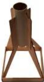
❑ 12. Test fit the Large Body Tube over the outside of the fins, making sure it fits in the slot in the fins. Sand the sides of the fins if necessary. Once you have the fins so the tube fits over them, apply glue and re-install the body tube. It should now look like the picture.
