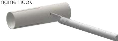
❑ 4. Insert one end of the engine hook (EH-28) in the slit.
