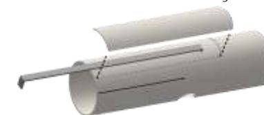
❑ 7. Press it into place, conforming with the engine hook. Clean up any excess glue and allow to dry.
