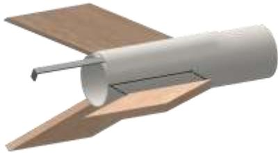
❑ 10. After the fin assembly is completely dry, run a small bead of glue along both sides of each fin-body tube joint. Using your forefinger, smooth the glue into fillets. Fit one of the fin tips on the root edge of a main fin. Place a small mark at the ring slot in the main fin. Repeat with the other two fins.
