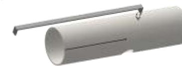
❑ 5. Run a bead of glue over the engine hook and about 1/8" on each side of the hook. Align the Tyvek strip over the engine hook with the rounded end toward the top and the flat end even with the bottom of the body tube.
