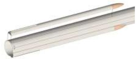
22. Glue the crew module on the main body tube along the set of lines drawn earlier on the opposite side from the LL line. Offset it 1/4" from the end of the main tube. Allow to dry.
