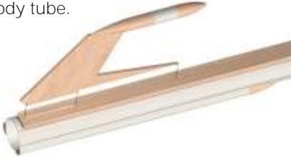
❑ 27. Apply glue to the root edge of one of the remaining completed pod assemblies and position it with the tab centered in the slot in the reactor bay. Remove the fin, set it aside and allow it to almost dry, apply additional glue, and reposition. Allow the fins to completely dry, checking carefully to make sure they are parallel with the main body tube. Repeat with the last pod assembly.
