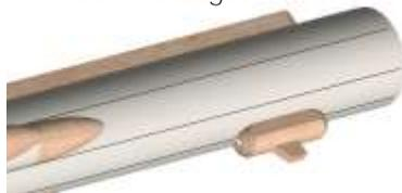
❑ 33. Glue the long launch lug (LL-140) on the LL line and even with the bottom of the main tube. Allow to dry.
