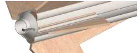
❑ 36. Apply a bead of glue to the small trailing edge of each main fin and attach a small wood dowel (WD-128) to each one. These are to reinforce the exposed edges. At this time, the long trailing edges and the leading edges of all the fins may be rounded or left flat.
