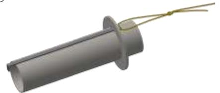
❑ 10. Wrap masking tape around the center of the engine tube to hold the engine hook in place and centered along its length. Run a bead of glue over the masking tape and along the engine hook between the tape and the ring. Allow to dry.
