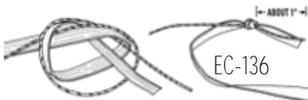
❑ 41. Assemble the 15" chute (CP-12-24) using instructions provided with it. Pull the lines tight on the chute and make sure they are all of equal length. Attach the chute by tying them to the screw eye. Put a drop of glue on the joint to keep the lines from moving. Attach the free end of the elastic cord to the screw eye. Put a drop of glue on that joint as well.
