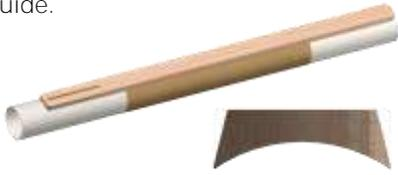
13. Cut one of the small nose cones (BNC-5E) into two identical halves. Using the sandpaper wrapped around the main tube, sand each half in a concave shape until the outside edges of the nose cone shoulder just touch the sandpaper.
