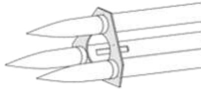
❑ 23. Slide the short slotted body tube assembly into the bottom alignment guide (with long nose cones) and line up the slots in the pod tubes with the slots in the large body tube. When the slots are aligned, place a mark at the small triangles on the alignment guide on the three pod tubes and the "L" on the large body tube. NO glue yet!
