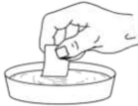
❑ 38. Slide the decal in place and use the paper backing to work the bubble out. Repeat for all the decals. Be careful with covering decals with a clear coat. Many of the new sprays are not compatible. Future floor polish is suggested.
