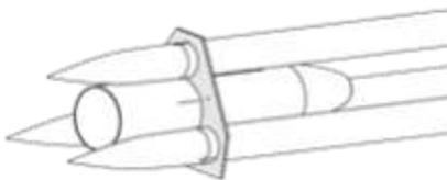
❑ 24. Slide the long slotted body tube assembly into the top alignment guide and line up the slots in the pod tubes with the slots in the large body tube. When the slots are aligned, place a mark at the "L" on the large body tube. NO glue yet!
