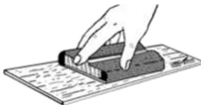
3. Stack all three fins in a group. Line the set of fins up squarely and sand the fins back and forth over some fine sandpaper to get rid of the hold-in tabs as shown below.
