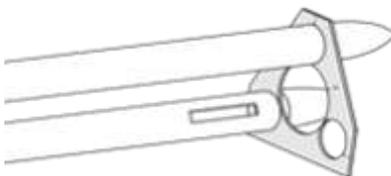
❑ 21. Add the third pod to the alignment guide and center its slot as the other tubes were centered. Place the alignment guide on a flat surface with the longest edge on the surface. NO glue yet!
