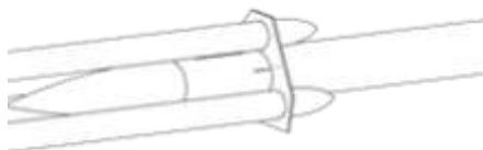
❑ 25. Check the entire assembly for alignment. Make sure the alignment guides are flat on the table. Make sure all the slots in the two large tubes are aligned with the corresponding slots in the pod tubes. When you are satisfied that everything is aligned, tack each pod tube to the larger tubes using a small amount of glue. Keep the glue away from the alignment guides. Allow the glue to dry.
