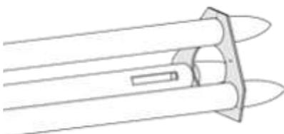
❑ 22. Carefully insert the three long nose cones into the second alignment guide. Make sure the **small "L" cut into the guide is aligned with the "L" in the first alignment guide.** This will be the mark for the launch lug in a later step. Slide the alignment guide until 1/8" is showing from the end of the tube to the alignment guide. NO glue yet!
