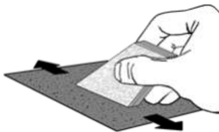
4. Round the leading, trailing and tip edges of each fin. Leave the root edges flat. The root edges will be glued to the body tube and nose cone.
