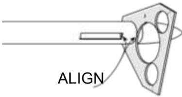
❑ 20. Insert the top of the second pod assembly into the alignment guide. Turn the tube until the slot in the tube is centered with the gap in the alignment guide. The top of the tube should be about 1/8" from the alignment guide. The two tubes should have the slots facing inwards. NO glue yet!
