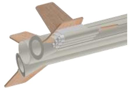
❑ 30. Repeat with the other ramjet assembly on the other wing. Check for alignment as shown below.
