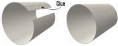
❑ 12. Apply a bead of glue around the inside rim of one of the complete shrouds. Fit one of the two centering rings (large hole) into the bottom of the shroud. Place the shroud with the ring down on some wax paper and make sure the ring is flat and the shroud touches the wax paper as shown in the cutaway view. Repeat with the other shroud and ring. Allow both assemblies to dry.
