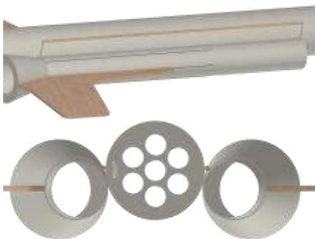
❑ 24. Apply glue to the root edge of one of the rudders and position it on the top line on one of the tank tubes and even with the top of the shroud. Use the alignment guide to get the correct angle. Use the same techniques used on the main fins. Repeat with the other rudder on the other tank tube. Allow both rudders to completely dry using the alignment guide to make sure they remain positioned correctly.
