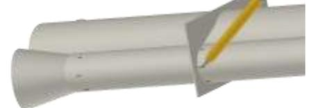
❑ 20. Using a straightedge or ruler aligned on the sets of marks, extend a line from the shroud for about 6' along the tank tubes. Extend the line on the top of the main tube for 7".
