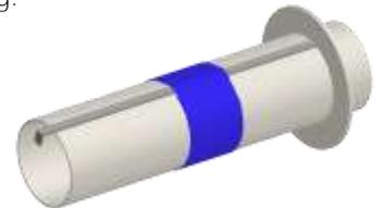
9. Slide the centering ring with the small holes and large notch over the bottom of the engine tube with the engine hook inside the notch. Run a bead of glue around both centering rings along the ring and tube joint, keeping glue away from the bottom engine hook notch.
