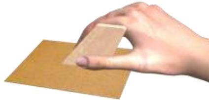
4. Round all the edges of each fin, except leave the root edges flat. The root edges will be glued to the body tube. There is one extra forward vane that will not be used.
