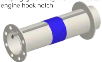
10. Glue the thrust ring (TR-9) in place on top of the engine hook as shown. Allow all the joints to dry.
