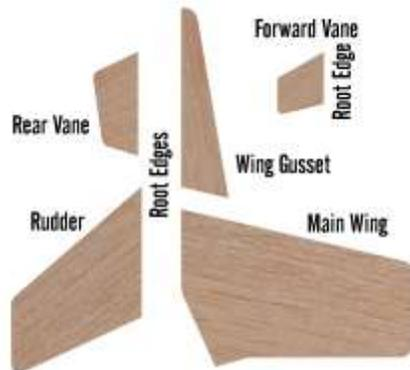
5. Glue each main wing and wing gusset as shown below. Use a straightedge or ruler to align the two parts along the root edges. Wax paper will prevent parts from sticking to your workspace.
