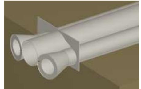
❑ 18. Position the template about 1/2" from the shrouds. Place a mark at each triangular cutout. There are three on each tank tube and one at the top of the main tube.
