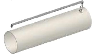
8. Carefully punch out all the fiber parts from the laser-cut fiber sheet (CR-KV-77). Slide the centering ring with the small notch over the engine tube and engine hook until the hook is just captured. Wrap one layer of masking tape around the center of the tube, holding the engine hook in place. Run a bead of glue along the engine hook from the tape to the top ring.
