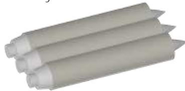
❑ 27. Glue three fiber ramjet supports to the ramjet tubes. Align them with the bottom edge of each support even with the bottom (nozzle) end of each jet tube as shown. Make sure they are all perpendicular to the body tube.
