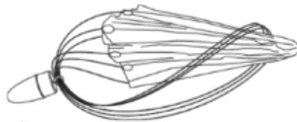
❑ 25. Tie the free end of the Kevlar shock cord to the screw eye.
