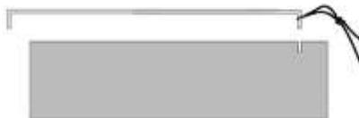
5. Pass the remaining length of Kevlar through the motor tube and out the bottom. Apply a ring of glue around the motor tube at the 1 inch mark and another just below the tube slot as shown.
