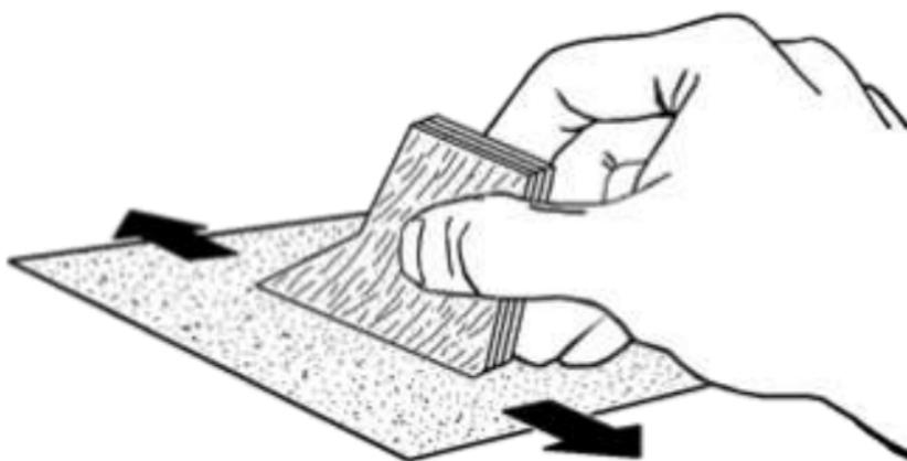
□ 13. Round all edges except the root edges (which will be glued to the body tube). Again, avoid sanding off the slight tab on the large fins.
