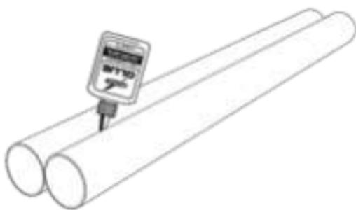
4. Stack the final engine tube on the other two and apply a bead of glue to each joint. Make sure the three marked ends are all in the same direction. This marked end is the bottom of the rocket. Allow this assembly to completely dry.
